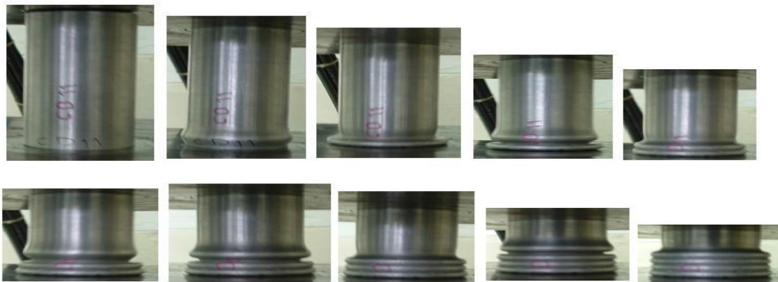
Fig.2. Typical deformation history of cylindrical shells under axial compression
