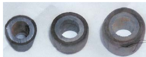
Fig 3 : Swelling elastomers. Original thickness: steel 4mm, rubber 3.6mm (left); 66% swelling (middle); 118% swelling (right), (Braas et al 2003).
