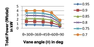
Fig.9: Total power output versus vane angles (vane numbers) at different rotor / casing (d/D) ratio when injection pressure = 6 bar and speed of rotation =2500 rpm
