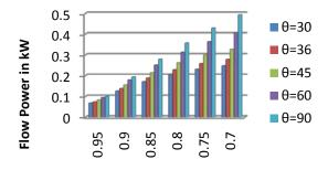
Fig.5: Exit flow power versus rotor / casing diameter (d/D) ratio at different vane number (vane angles) when D=100 mm, injection pressure = 6 bar and speed of rotation =2500 rpm.
