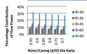
Fig.7: Percentage contribution of exit flow power versus rotor / casing diameter (d/D) ratio at different vane number (vane angles) when D=100 mm, injection pressure = 6 bar and speed of rotation =2500 rpm
