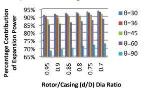
Fig.6: Percentage contribution of expansion power versus rotor / casing diameter (d/D) ratio at different vane number (vane angles) when D=100 mm, injection pressure = 6 bar and speed of rotation =2500 rpm
