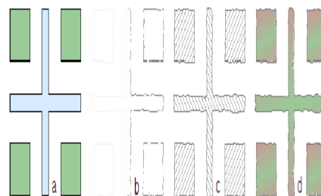
Figure 4 : schematic drawing of polymeric alignment marks and their microscope images. a) mark as designed, b) left half: very weak contrast as obtained with standard reflected light illumination, right half: stronger contrast with transmitted light. Still the pattern is not ideally suited for pattern recognition due to its narrow contrasted structures. c) internal surface patterning of the target to enhance contrast and create expanded structures d) contrast as obtained with DIC
