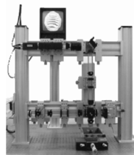
Figure 11 : Twyman-Green Interferometer for measuring surface deviations and radius of curvature.
