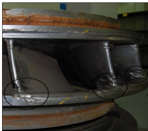
(a) Erosion at runner outlet
