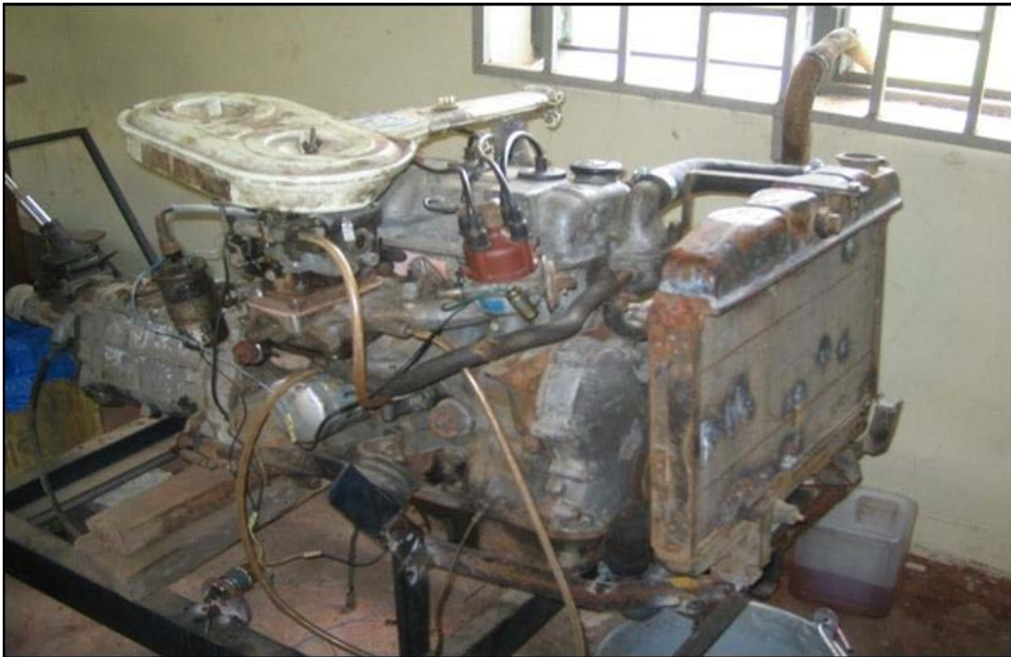
Figure 1 : Experimental rig: Toyota Carina II engine
