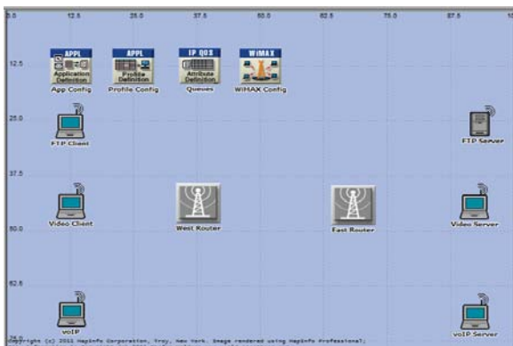
Figure 5: WiMAX network scenario with QoS
