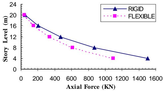
FIG10- Axial forces of C4 in Rectangular building with shear walls under X-X direction earthquake
