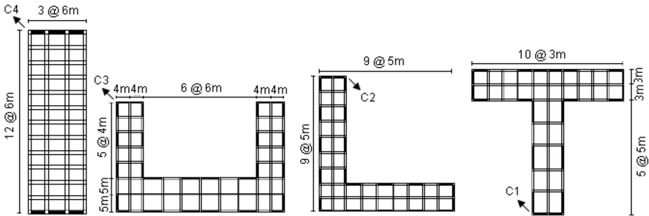
FIG. 3 Plan shape and position of shear walls
