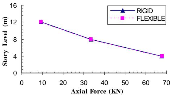
FIG 5- Axial forces of C1 in T-shaped building with shear walls under Y-Y direction earthquake
