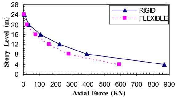
FIG. 7. Axial forces of C3 in U-shaped building without shear walls under Y-Y direction earthquake
