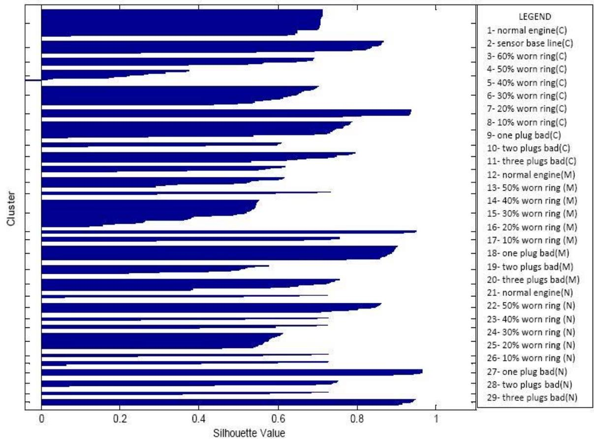
Figure 9: FCM silhouette diagram for the three engines
