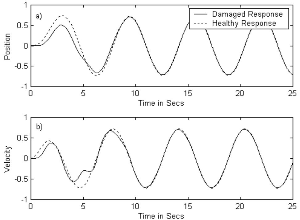
Figure 1: An Adaptation Law for Structural Damage Mitigation with Healthy and Damaged Responses a)  $y(t)$  and  $y_m(t)$  and b)  $y(t)$  and  $y_m(t)$
