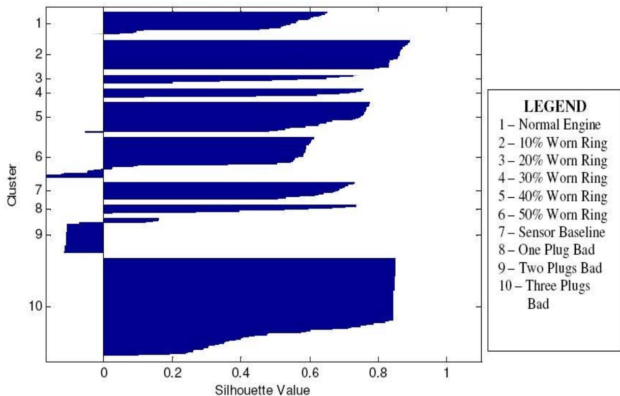
Figure 5: FCM silhouette diagram for Mitsubishi Gallant engine
