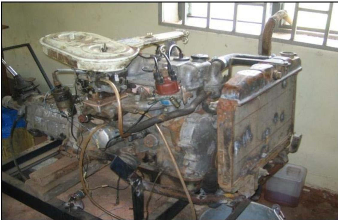
*Figure 1:* Experimental rig: Toyota Carina II engine
