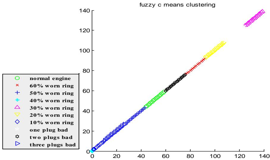
Figure 2: FCM diagram for Toyota Carina II engine
