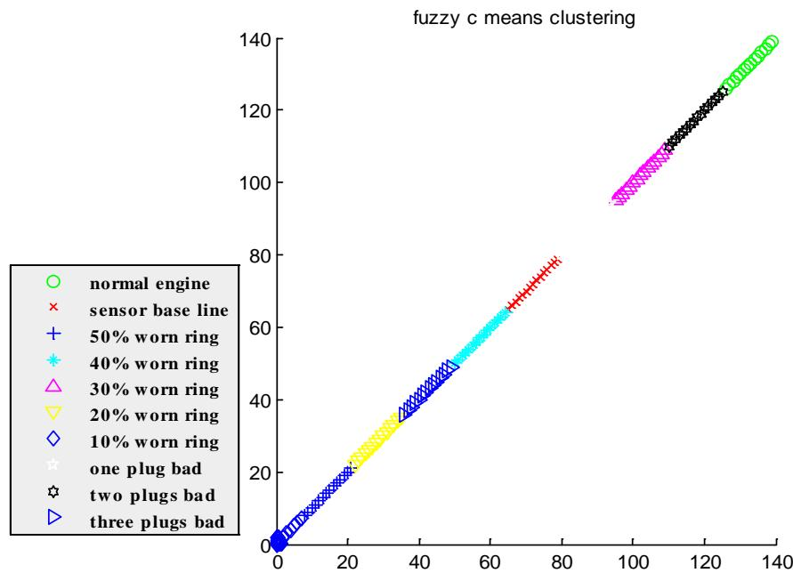
Figure 4: FCM diagram for Mitsubishi Gallant II engine
