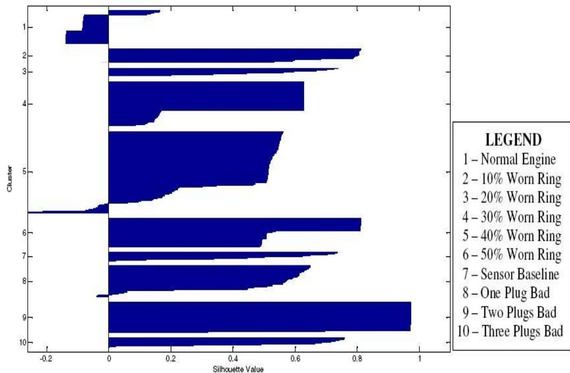
Figure 7: FCM silhouette diagram for Nissan Sunny engine
