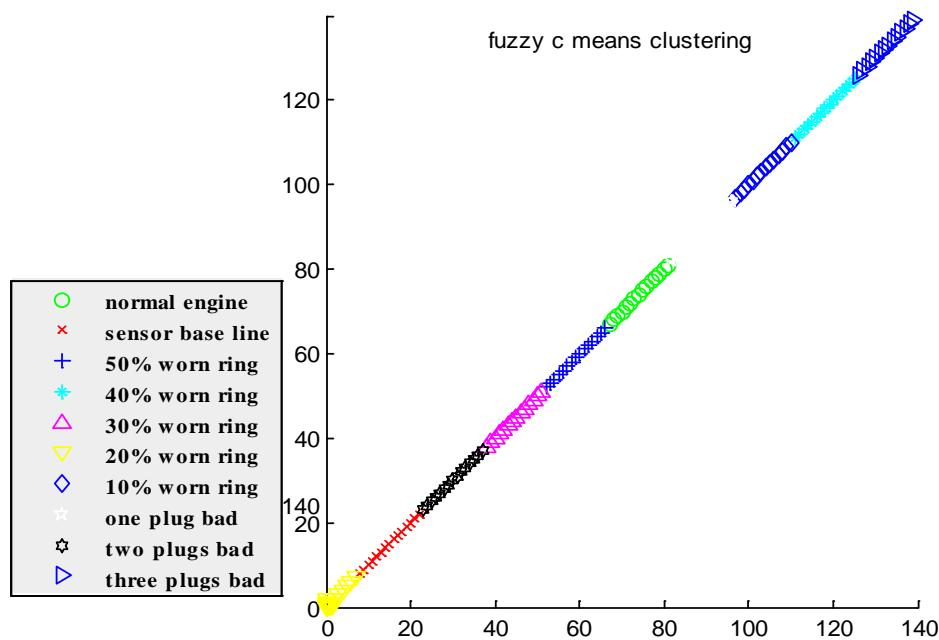
Figure 6: FCM diagram for Nissan Sunny engine
