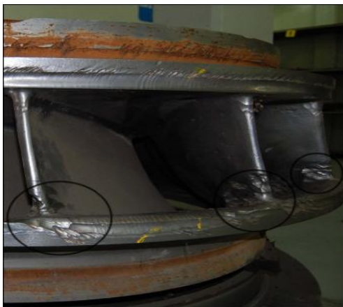
(a) Erosion at runner outlet
