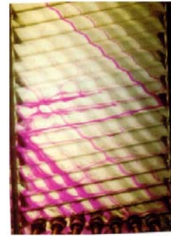
Figure 11.b) Flow visualization by Focke & Knibbe[7], Re=125
