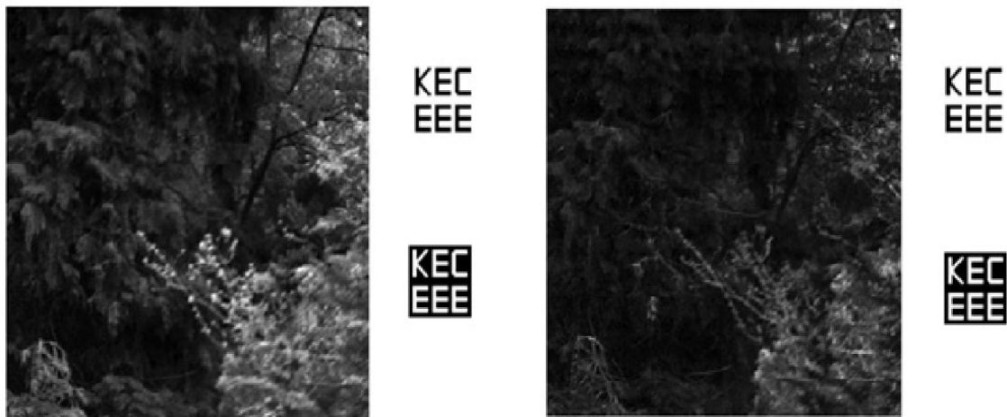
Figure 6 : (a) Host image (b) Original Watermark (c) Watermarked Image (d) Extracted Watermark
