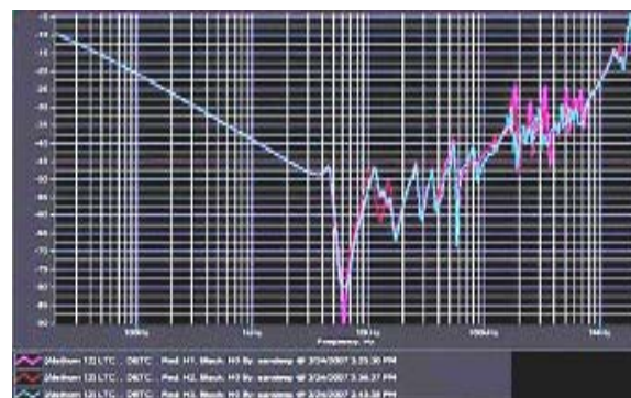
Figure 12 : HV winding response (LV short)
