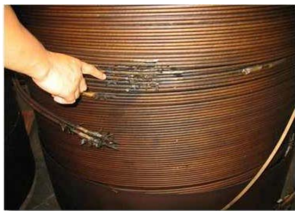
Figure 10 : Damaged LV (phase-C) coil
