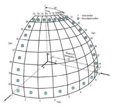
MacNeal and Harder (1985) indicates that the theoretical lower bound for the displacement at the point
