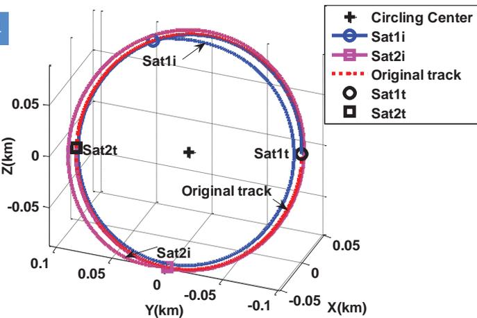
Figure 5 : Propagation of the phase angle adjustment.
