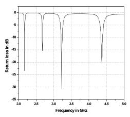
Fig. 4: Simulated return loss of the antenna2
