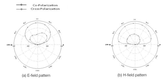
Fig. 8: Simulated normalize radiation pattern at 4.37 GHz
