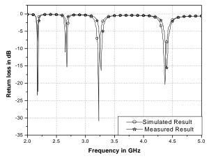
Fig. 10: Comparison between measured and simulated return losses for antenna 2
