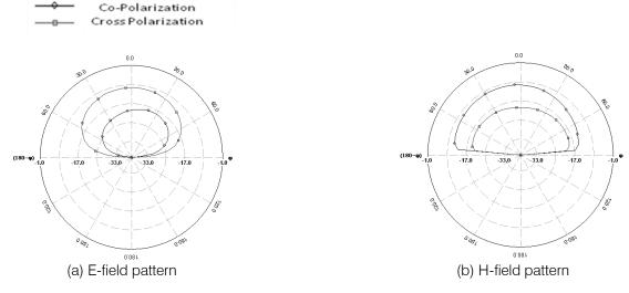
Fig. 6: Simulated radiation pattern at 2.68 GHz
