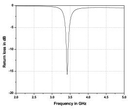
Fig. 3: Simulated return loss of the antenna1
