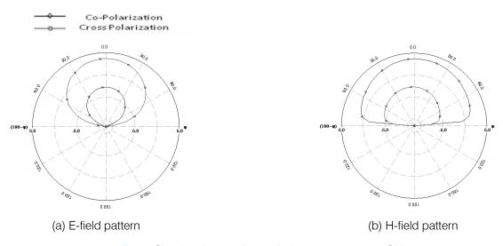
Fig. 7: Simulated normalize radiation pattern at 3.22 GHz
