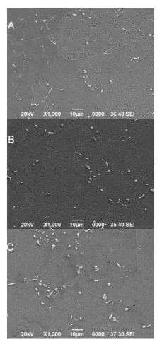
Fig. 9: Photograph of SEM result welded specimen heated at A) 200 °C, B) 400°C and C) 600°C, Etched by Kalling Reagent's no. 2, 1000x
