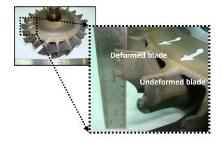
Fig. 2: Failed and worn out turbine wheel blade tip due to cracking, two samples of defomed and undeformed blade were researched
