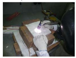
Fig. 5: GTAW process being performed
