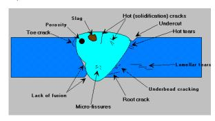
Fig. 1: Types of defects on weldments (Fontana, F.G., 1987)
