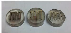
Fig. 7: Photographs of prepared specimen for metallographic examination
