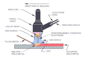
Fig. 4: Schematic of GTAW Technique (http://www.spectroweldinstitute.com)
