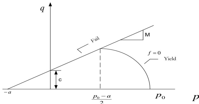
Figure 9: Cam Clay Cap Model
