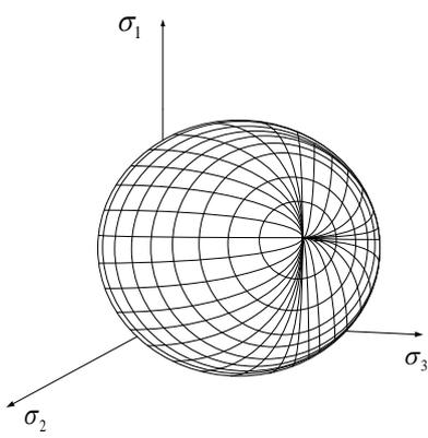
Figure 7: Cam Clay Failure Criterion in the Deviatoric Plane
