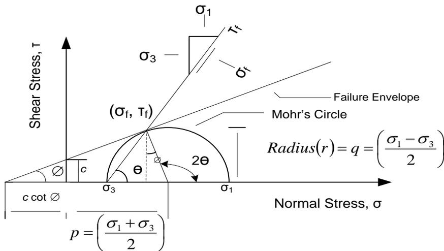
Figure 6 : Mohr-Coulomb failure criterion
