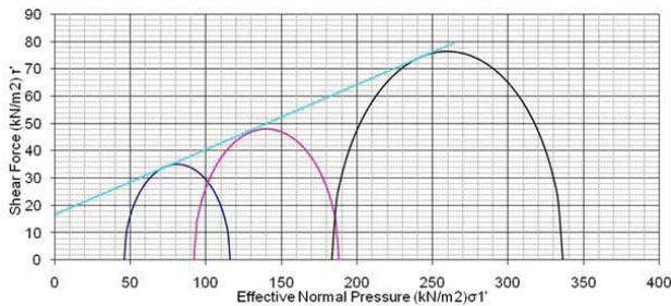
Figure 12 : Mohr-Coulomb failure envelope for non treated expansive soils
