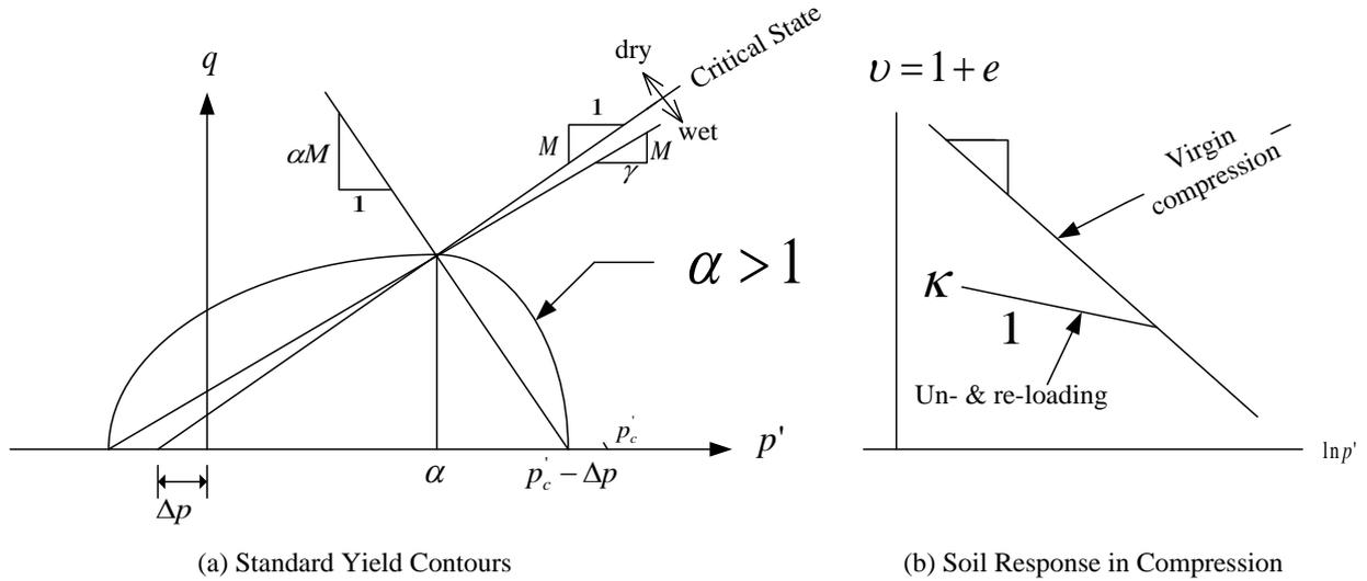
Figure 10 : Egg Cam Clay Models
