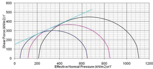
Figure 13 : Mohr-Coulomb failure envelope for 4% lime treated expansive soils
