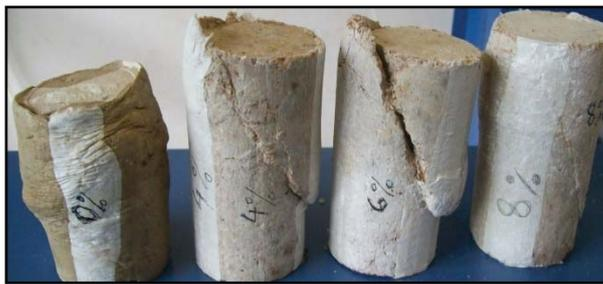
Figure 11 : Triaxial compression (CU) samples after test
