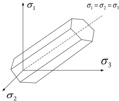
Figure 1 : Tresca Yield Criterion (Maximum-Shear-Stress Failure Theory)
