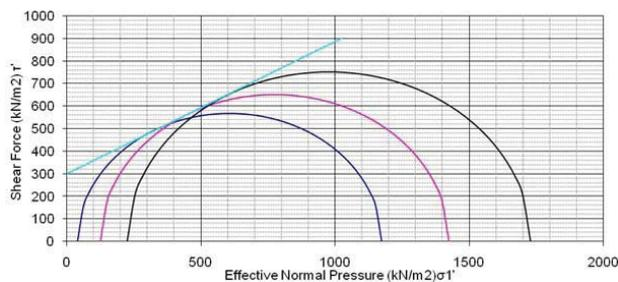
Figure 14 : Mohr-Coulomb failure envelope for 6% lime treated expansive soils
