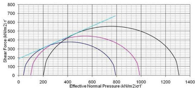
Figure 15 : Mohr-Coulomb failure envelope for 8% lime treated expansive soils
