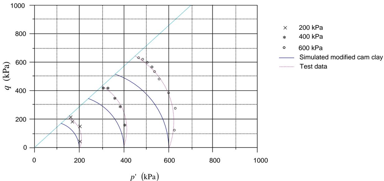
Figure 16 : Comparison between simulated modified cam clay model and test data for 6% lime treated expansive soil
