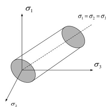
Figure 2 : von Mises Yield Surface in Principal Stress Space (Distortion Energy Theory)
