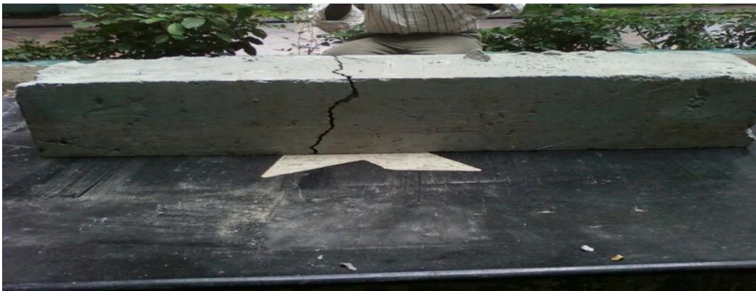
Shear failure of Plain S.S.C beam
