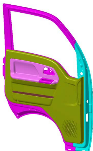
Fig 2 : Assembly of molded trim and with inner panel
