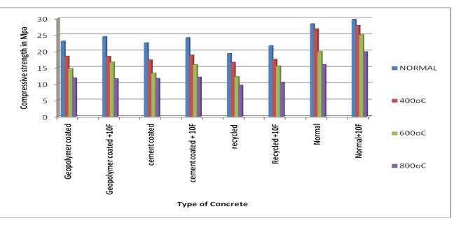
*Fig 4*: Cube compressive strength of natural aggregate concrete and concrete out of coated recycled aggregate concrete ( with and without flyash)
