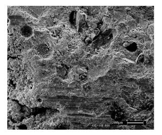
*Fig 8*: Microstructure of Geo polymer coated RAC -10F sample after exposing to 800°C temperature
