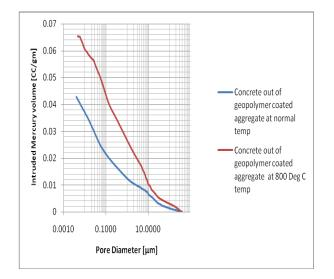
*Fig 2*: Comparison of intruded mercury volume vs pore diameter curve for concrete out of geopolymer coated aggregate at normal temperature and after heating to 800°C temperature
