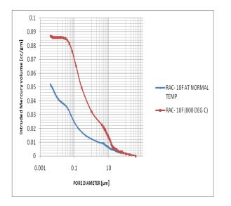
*Fig 1* : Comparison of intruded mercury volume vs pore diameter curve for recycled aggregate concrete with 10% fly ash at normal temperature and after heating to 800°C temperature<sup>[4]</sup>
