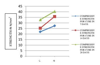
*Figure 5* : Compressive strength of M30 grade concrete cubes
