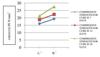
Figure 4 : Compressive strength of M20 grade concrete cubes
