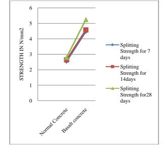
Figure 7 : Split tensile strength of M30 grade concrete
