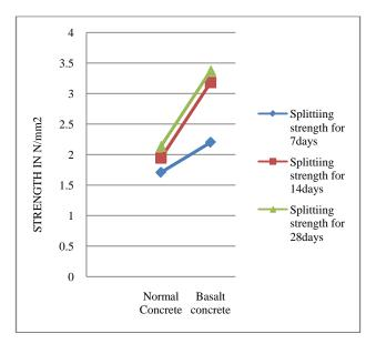
Figure 6: Split tensile strength of M20 grade concrete
