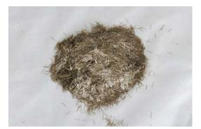
Figure 1 : Basalt fibre
