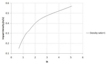
Fig. 9: The particle impact velocity with the bend surface for different Stokes number considering the density ratio is bigger than one
