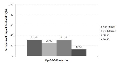
Fig. 6: The particle impact probability at different area of bend wall by changing the particle diameter
