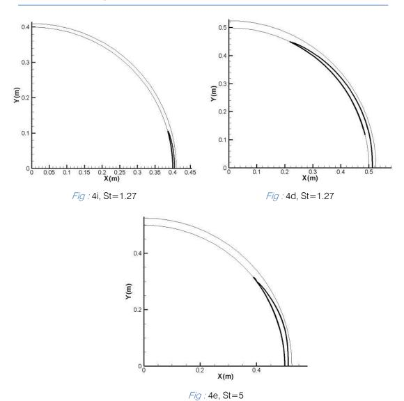
Fig. 4: Particle movement path inside the bend for different Stokes number of 0.34, 0.78, 1.1, 1.27 and 5; a, b, c, d and e for air and f, g, h and i for water
