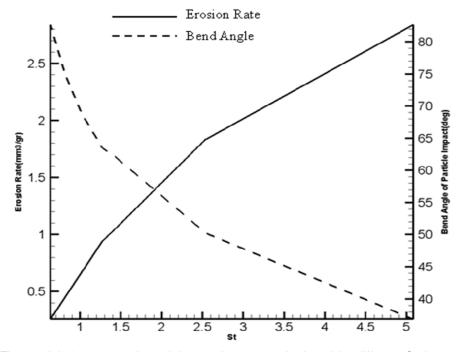
Fig11: The particle impact angle and the erosion rate at the bend for different Stokes number
