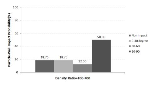
Fig. 7. The particle impact probability at different area of bend wall by changing the density ratios
