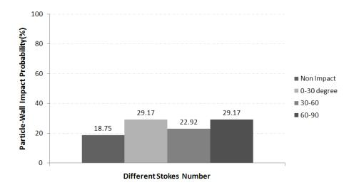
Fig. 8: The particle impact probability at different area of bend wall for different Stokes number
