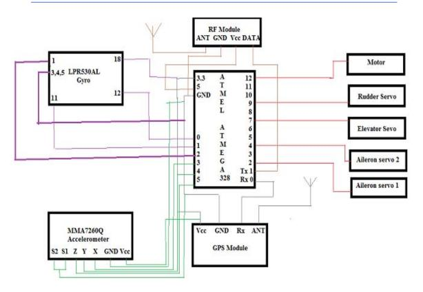
Fig 1 : Block diagram representation of UAV
