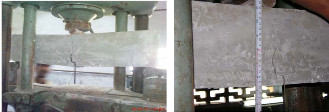
Figure 4 : Mode of failure and crack pattern of all the beams tested
