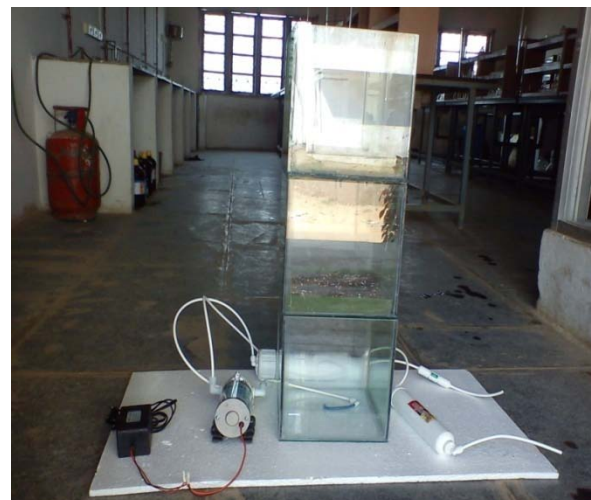
Fig. 3.3.3 : Rapid sand filter with RO.
