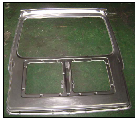
Fig.2 : A completed panel after press work
