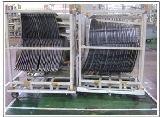
Fig.1 : Shows the cutout panels are stacked properly together in a trolley in order to maintain 5-S culture.
