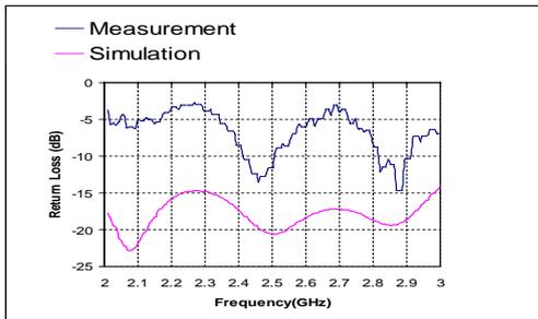
Figure 17: Simulated and measured return loss versus frequency
