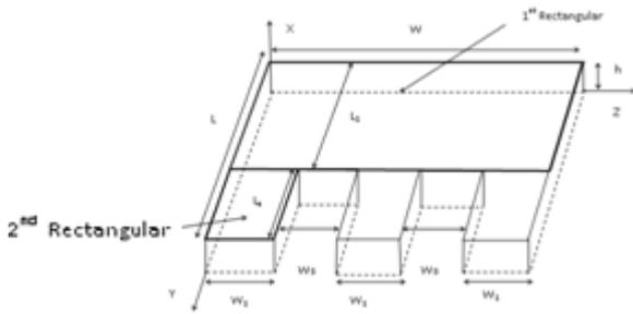
Figure 3 : E-shape microstrip antenna
