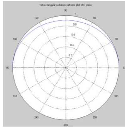
Figure 6 : Radiation pattern of 1<sup>st</sup> rectangle E-plane
