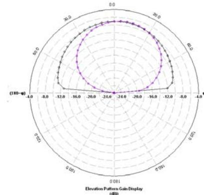
Figure 16 : Radiation pattern of E-shape microstrip antenna
