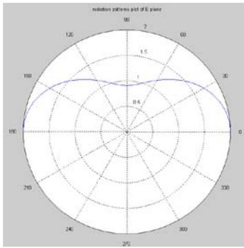
Figure 10 : Radiation pattern of E-shape microstrip antenna (E-plane)
