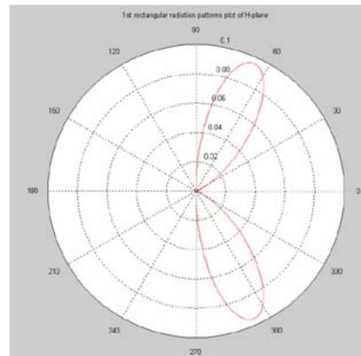
Figure 7 : Radiation pattern of 1<sup>st</sup> rectangle H-plane
