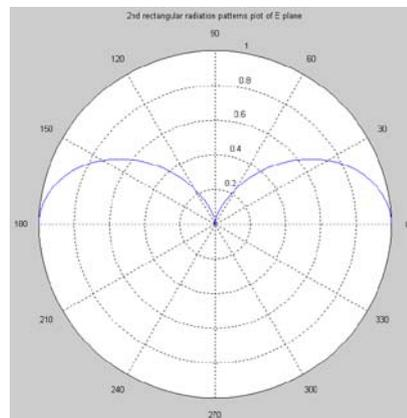
Figure 8 : Radiation pattern of 2<sup>nd</sup> rectangle E-plane
