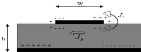
Figure 1 : Charge distribution and current density creation on the patch.
