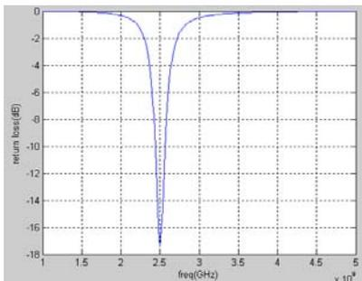
Figure 5 : Return loss of E-shape microstrip antenna
