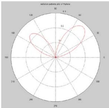
Figure 11 : Radiation pattern of E-shape microstrip antenna (H-plane)
