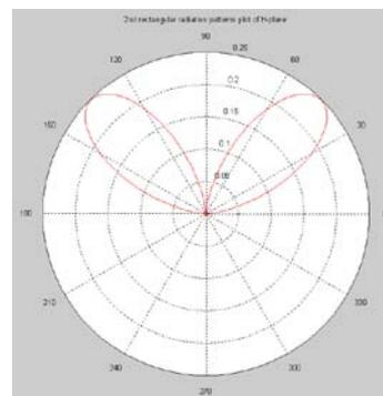
Figure 9 : Radiation pattern of 2<sup>nd</sup> rectangle H-plane
