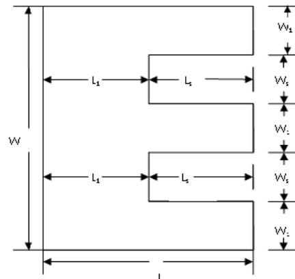
Figure 2 : Geometry of proposed E-shape antenna
