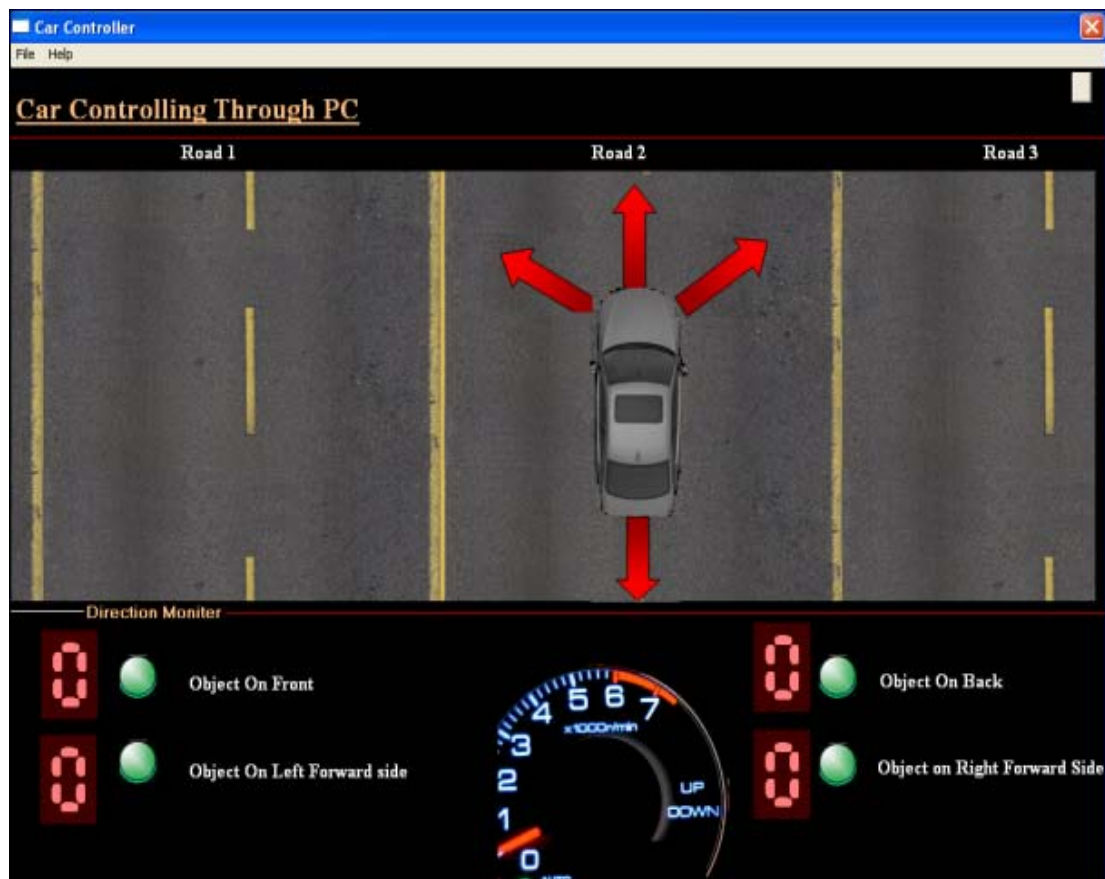
Figure.7 : Distance Measuring interface on PC (Software)
