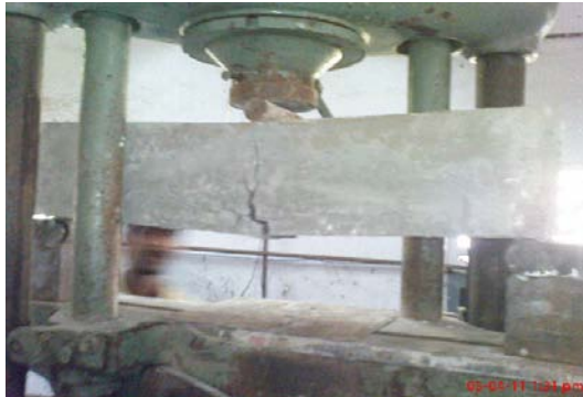
Figure 4 : Mode of failure and crack pattern of all the beams tested
