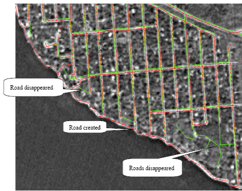
Figure 10 : Road centerlines extracted from IRS pan image of urban area (red dashed line) superimposed with NTDB roads (green solid line)
