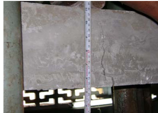
Figure 4 : Mode of failure and crack pattern of all the beams tested
