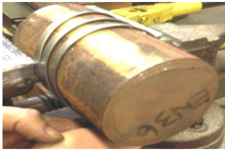
Figure 2 : Experimental simulation of reverse bending of tensile armour bar
