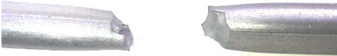
(b) Fractured experimentally RBS specimen.
