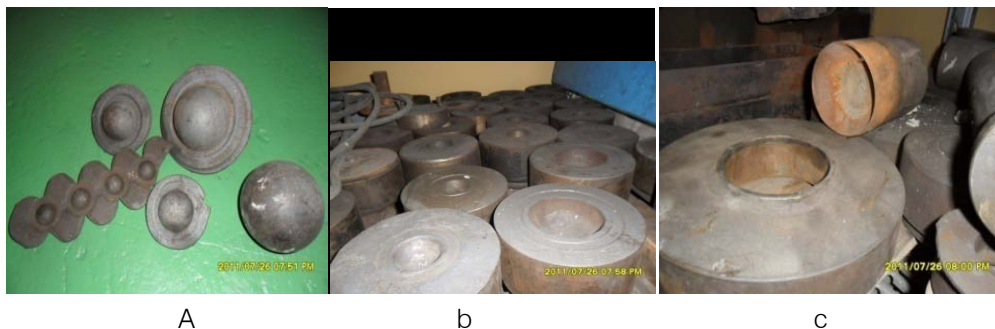
Fig. 4 : a) steel balls b) steel ball forging dies c) trimming dies; photo from Akaki Basic Metals Industry
