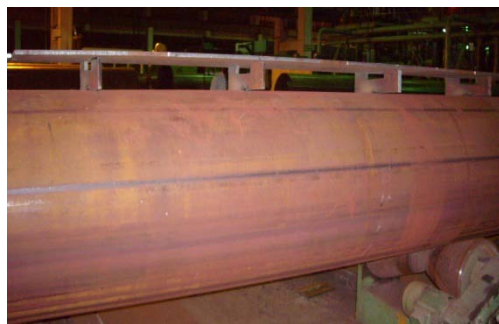
Figure 2 (a) : Weld Test Coupon Assembly, (b) Double-V joint geometry for Test Coupon
