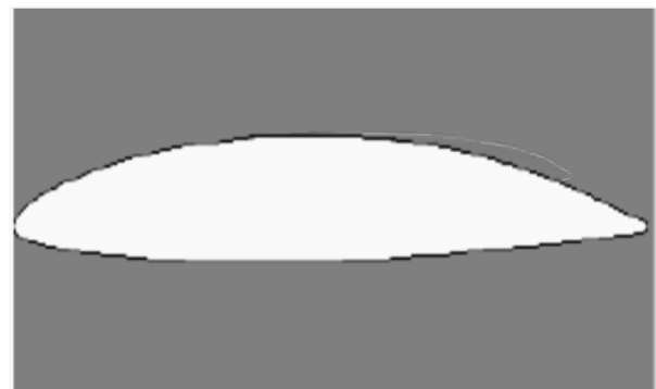
Figure 1 : Cavity at the mid-chord region
