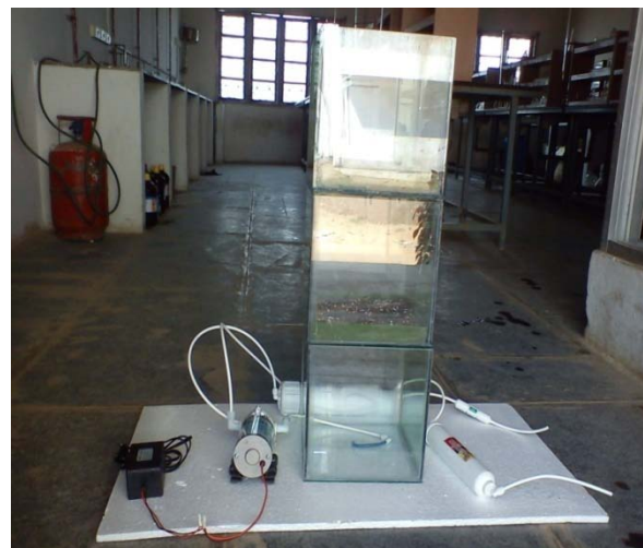
Fig. 3.3.3 : Rapid sand filter with RO.
