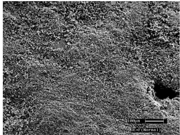
Fig 7 : Microstructure of Geo polymer coated RAC -10F sample before exposing to 800°C temperature
