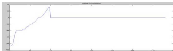
Fig10 : Level-2 Wavelet Decomposed ST-Segment of Normal ECG signal.
