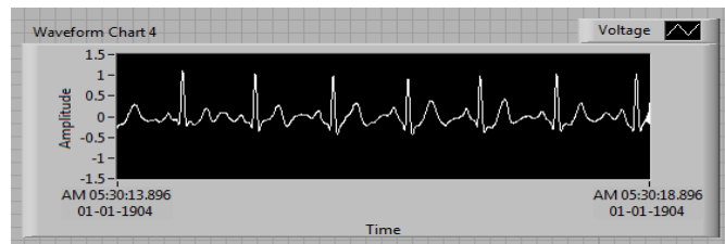
Fig 14 : ECG signal after baseline correction and noise removal
