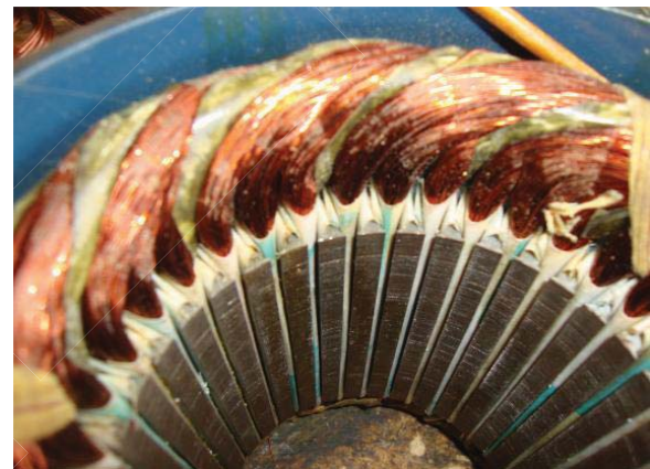
Fig.9 : New induction motor
