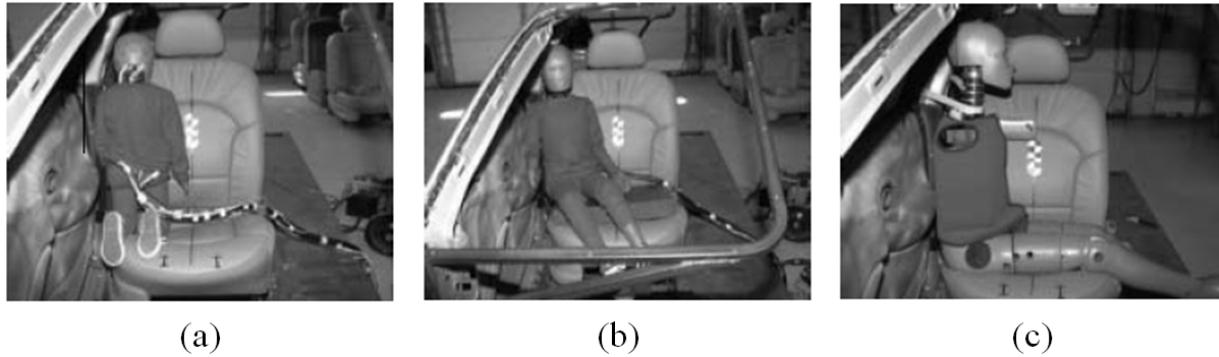
Figures 1 : OOP test configurations [7].
