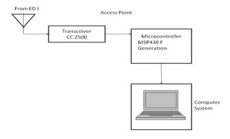
Figure 2: Block diagram for access point
