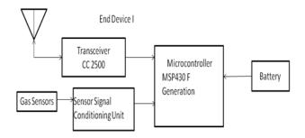
Figure 1: Block diagram for end device
