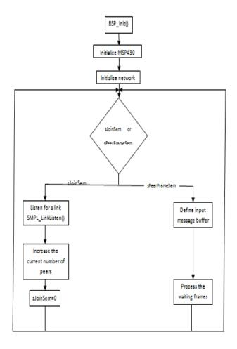
Figure 3: Algorithm for Access Point
