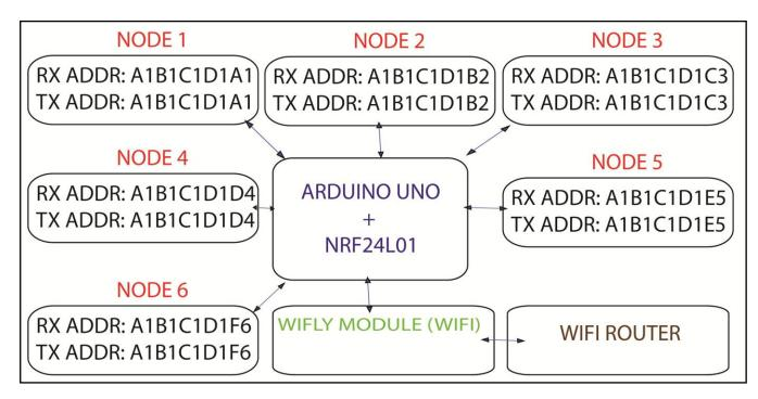
Figure 6: Mesh networking of 6 nodes with base station
