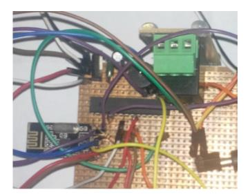
Figure 11: Control Node to control Machines
