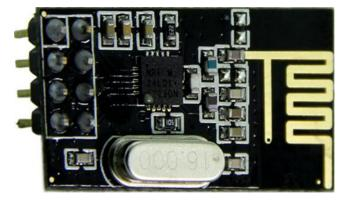
Figure 4: NRF24L01 Transceiver
