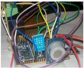
Figure 13: Sensing Node for sensing temperature and humidity
