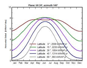
*Figure 4 :* Monthly Horizontal global radiation for different latitudes in Dhaka
