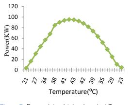
*Figure 7:* Power data obtained against Temperature when Tilt/Azimuth is 1<sup>0</sup>/0<sup>0</sup>
