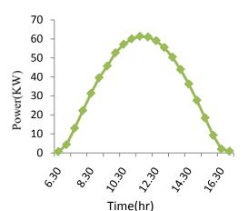
*Figure 10 :* Power data obtained against Time when Tilt/Azimuth is 21<sup>0</sup>/180<sup>0</sup>
