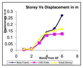
Figure 2: Story Level Vs Displacement Curve
