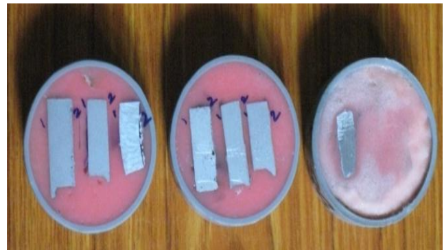
Figure 3 : Machined specimen for microstructure
