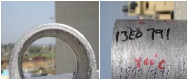
Figure 2 : Castings of 8 mm-thick cylinders
