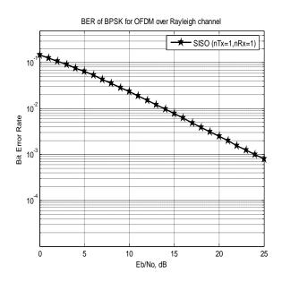
*Figure 5* : BER of SISO-OFDM system over Rayleigh Fading Channel
