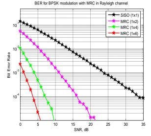
*Figure 7(b) :* BER for OFDM with MRC (SIMO-OFDM) in Rayleigh Fading Channel
