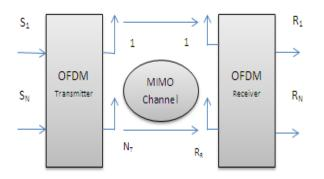
Figure 2 : MIMO-OFDM System Model
