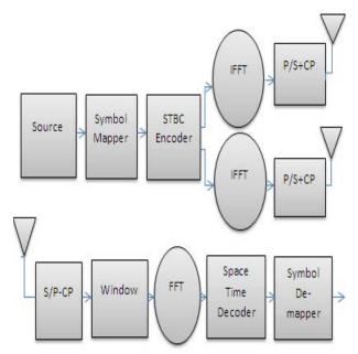
Figure 3 : Alamouti Coded OFDM System Model
