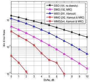
*Figure 8* : BER for MIMO-OFDM with Alamouti STBC and MRC Diversity over Rayleigh Fading Channel
