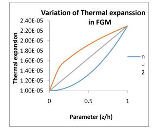
*Figure 4 :* Variation of effective Thermal expansion with respect to parameter z/h for various material index
