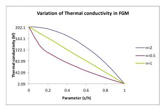
*Figure 3* : Variation of effective Thermal conductivity with respect to parameter z/h for various material index
