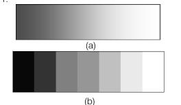
*Figure 1 :* Gradient of FGMs; (a) continuously graded and (b) discretely layered FGMs
