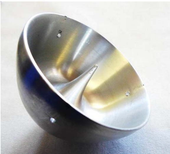
Figure 2 : An interior-exterior view of the parabolic deflector
