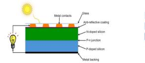
Figure 1 : Basic structure of a silicon solar cell. [3]
