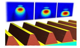
*Figure 3*: Sawtooth Tapered ridges, made from alternating layers of metal and insulating material deposited on a surface, can produce a metamaterial that is tuned to a range of specific frequencies of light. Light of different wavelengths is absorbed by the material at different levels, where the light's wavelength matches the width of the ridges. Designed in MIT's Department of Mechanical Engineering
