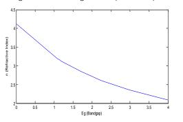
Figure 4: Typical band gap vs refractive index Curve
