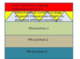
*Figure 8 :* Proposed metamaterial solar cell, where P-N junction can be normal or composite metamaterial
