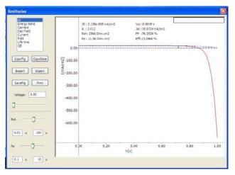
Figure 13 : Cds – CdTe metamaterial solar cell I-V curve
