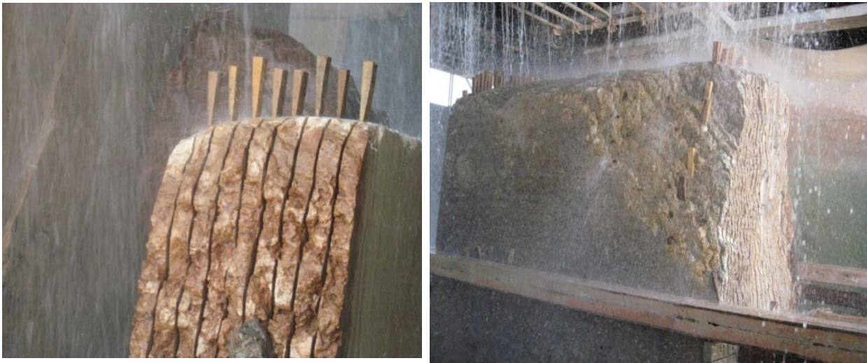
Figure 4 : Primary Cut Worksite
