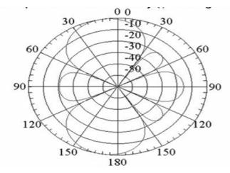
Figure 4 (d) : Directivity of "Antenna 3" in terms of Radiation Pattern
