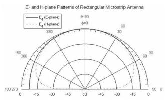
*Figure 4 (d) :* EH-field of "Antenna 3" in terms of Radiation Pattern
