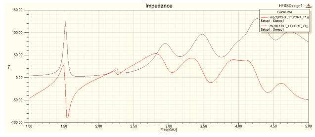
Figure 2 (c) : Impedance vs. Frequency curve of "Antenna 1"
