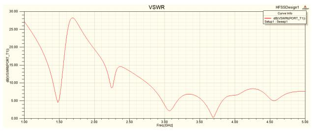
Figure 2 (b) : VSWR vs. Frequency Plot of "Antenna 1"
