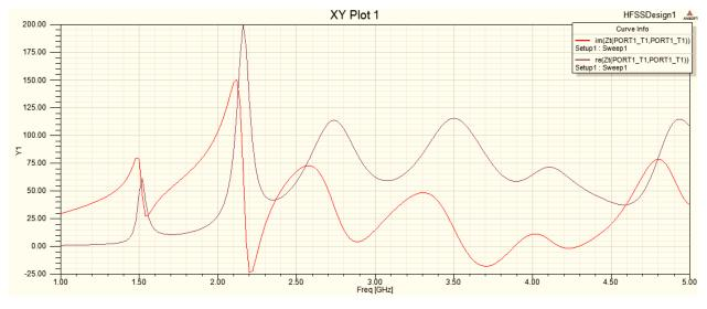
Figure 3 (c) : Impedance vs. Frequency curve of "Antenna 2"
